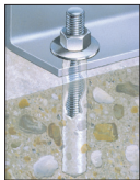
Fastening to Concrete with Threaded Rod
